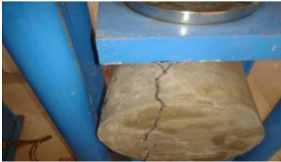
Figure 6.6 Cracking of concrete cylinder
