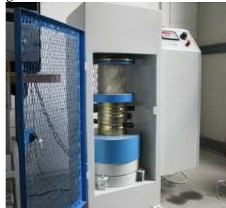
Figure 6.1 Compressive strength test of concrete
