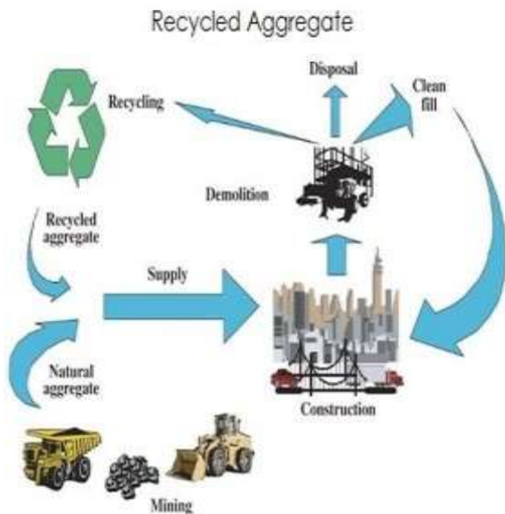
Figure No: 5.5 Processing of recycled concrete aggregate
